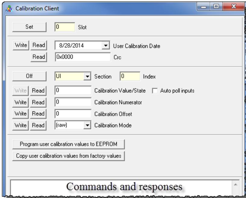
When read or write buttons are clicked, the program sends commands the controller. The controller responds to the program, and these commands and responses show up in the bottom area of the program. Updates to this area are automatic and there is no user input required.
