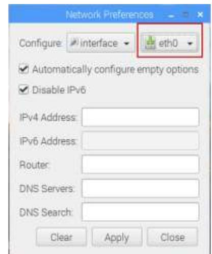
If you want the HMI panel to automatically obtain the network settings from a DHCP server on your network (the controller can act as such a server if enabled), then **check** the “Automatically configure empty options” and leave the “Disable IPv6” box checked.
