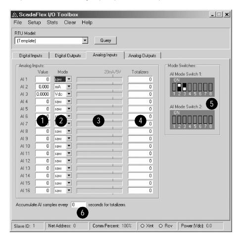
Most ScadaFlex I/O modules with analog inputs support multiple software selectable input modes; raw, current (20mA) and voltage (5Vdc). The raw mode is the "raw" uncalibrated, unscaled readings from the Analog to Digital converter circuitry in the module. In contrast, the current and voltage readings are calibrated and scaled.
