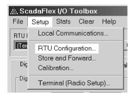
Each I/O module has non I/O type configuration parameters that may be viewed and set using the ScadaFlex I/O toolbox.
