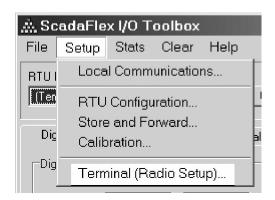
ScadaFlex RTUs are available with a built-in spread spectrum radio. The radio can be configured via a terminal emulator screen in the ScadaFlex I/O toolbox.
