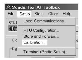
The inputs and outputs of analog I/O modules, as well as the power monitor of all modules can be calibrated using the ScadaFlex I/O toolbox.
