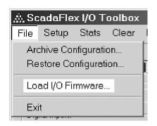
Before attempting to load new firmware into an I/O module, be sure that your PC is connected and "talking" to it.
