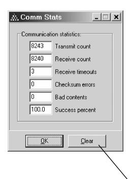
Statistics are kept continually as the Toolbox communicates with an I/O module. To clear existing values, for example, after connecting to a new unit, click on the "CLEAR" button.
