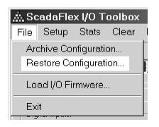
To restore a module configuration from a previously saved archive file, click on "File" on the upper menu bar, and then "Restore Configuration" in the menu that pops down. This will bring up a separate Windows "File Load" screen similar to the one pictured below:
