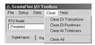
The Toolbox provides a facility for clearing the totals in groups or all at once. To access the totalizer clearing menu, click on "Clear" on the upper menu bar, and then "Clear DI Transitions", "Clear DI Runtimes", "Clear Al Totalizers" or "Clear All". The selected group of values will be set to zero.
