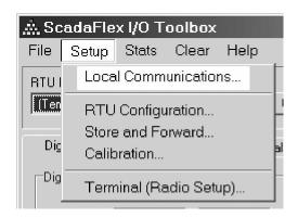
The "target" I/O module must be connected to the serial port of your PC computer and the Toolbox software must have several parameters set properly to communicate with a ScadaFlex I/O module.
