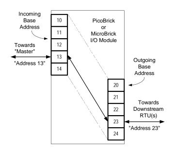
When the I/O module receives a message to be repeated, it translates the address, recalculates the checksum, and sends out the "new' message.
