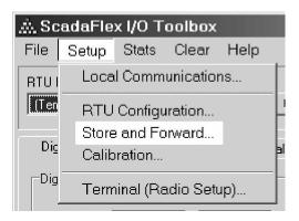
Each I/O module can serve as a Store and Forward digital message repeater for messages destined for other modules. This is typically used in wireless systems to effectively extend their coverage area.
