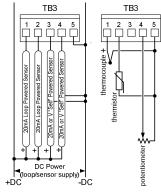
The optional universal analog inputs on terminal block 4 share a common that is isolated from all other I/O points. These inputs support 20mA and voltage signals, as well as 2-wire sensors (RTDs are not supported).
